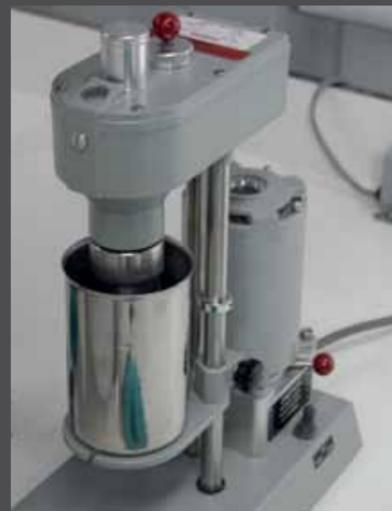
With the Fann Viscometer 35 SGS INTRON can accurately survey the viscosity of viscous fluids and slurries over a wide measuring range. With these data SGS INTRON can then determine the flow behaviour and, in consultation with the customer, give advice to improve it. Measurements are in accordance with API Recommended Practice 10B and viscosity levels up to 2500000 cP (centipoise) can be determined.
